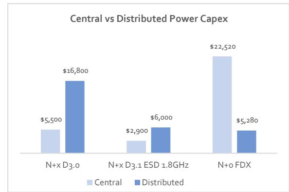
The above charts show the clear benefit of the Central powering approach in all cases except the significantly higher Capex cost associated with coax feeder upgrade when upgrading to a fiber-deep (N+o) configuration.
